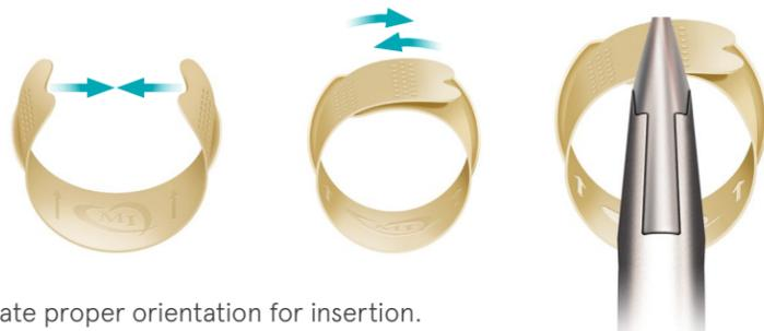
Directional arrow markers indicate proper orientation for insertion.
